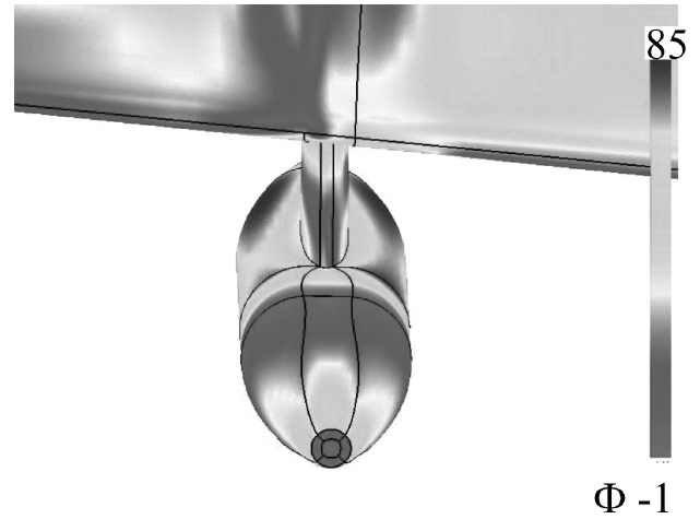
Fig. 2 Preprocessing—control of mesh orthogonality at the skin.
